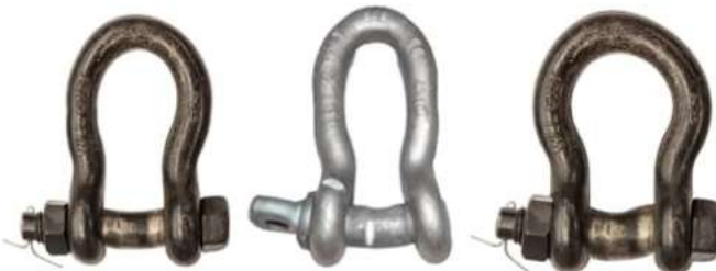
Bent, twisted, distorted, stretched, elongated body & pin
